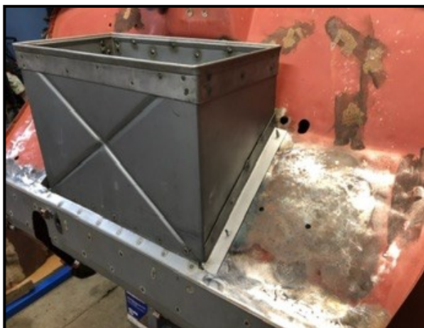
Fabricated new battery box firewall and sills.
