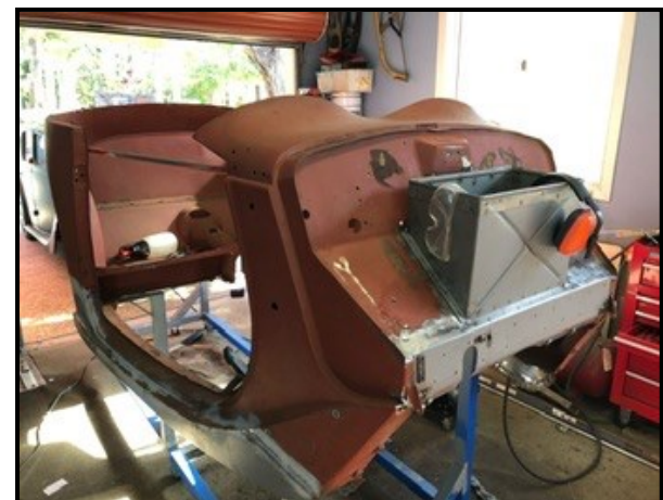
Fabricated new battery box firewall and sills.
