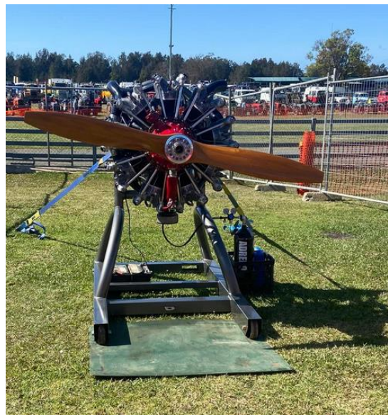
Vedeneyev M14P 360 hp (10 litre) radial as used in Yak 52 aircraft and many others
